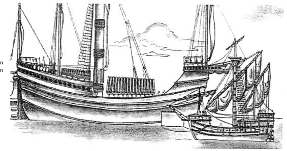
The small carrack is similar to the previous one, though its hull has about the same dimensions as the cogs. These carracks are common, both as traders and as warships. The cargo capacity is smaller than for a cog of the same size, but maneuverability and endurance are better.
